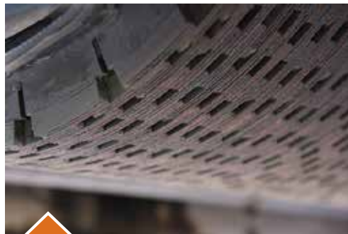
A close up of blades in Husqvarna’s Optimal Texture for City Streets (OTCS) concrete grinding system. The OTCS system is designed for lower-speed applications for traffic traveling up to 45 mph.
